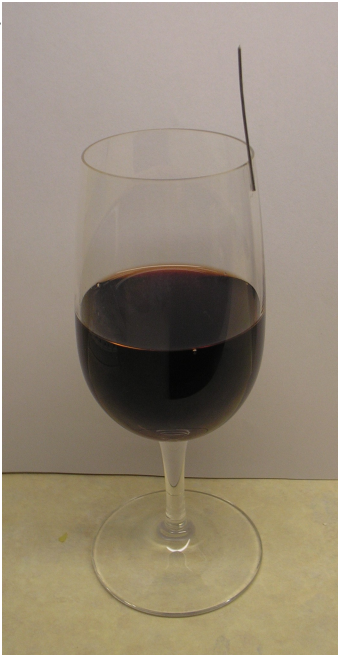
Figure 8: A tuned absorber on a wine glass (see http://www2.eng.cam.ac.uk/~hemh/tmd.htm )
